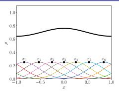
Density profile is expressed by the summation of the density profiles of SPH particles.
