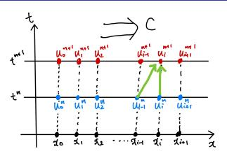
$$u_i^{n+1} = u_i^n - \frac{c\Delta t}{\Delta x} \left( u_i^n - u_{i-1}^n \right)$$
