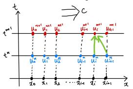
$$u_i^{n+1} = u_i^n - \frac{c\Delta t}{\Delta x} \left( u_{i+1}^n - u_i^n \right)$$
