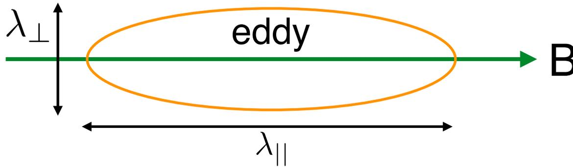
➔  $\frac{\lambda_{\parallel}}{l} \sim \left(\frac{\lambda_{\perp}}{l}\right)^{2/3} \left(\frac{v_l}{c_A}\right)^{-4/3}$  : MHD turbulence
